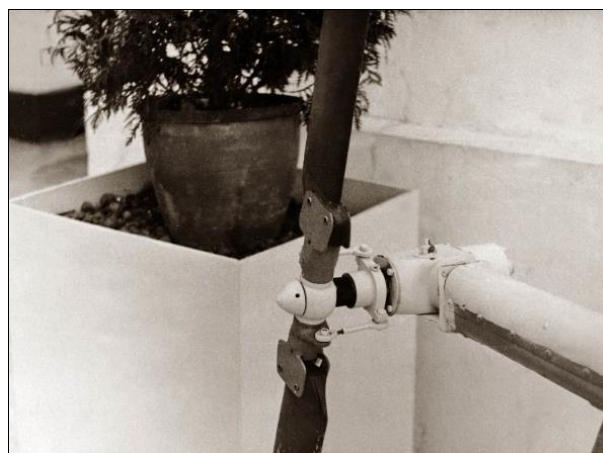
Tail rotor and its gearbox of the KhAI-27 Kharkovyanin helicopter.
