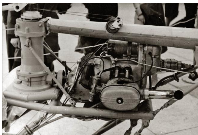
Powerplant and main rotor gearbox of the KhAI-27 Kharkovyanin helicopter. (Photo from the archive of Mr K. S. Gorbenko)
