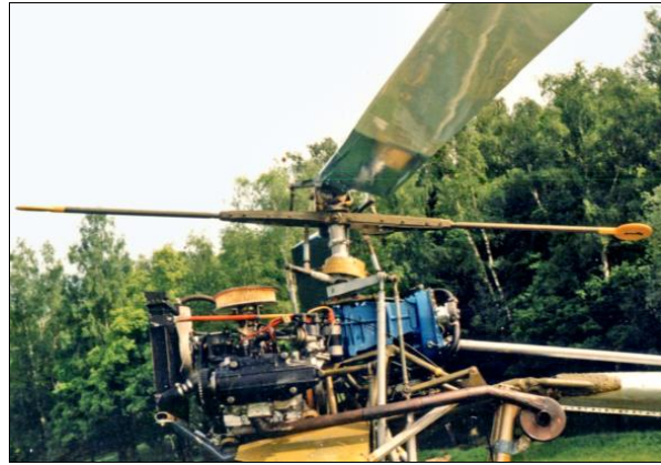
The powerplant and main rotor pylon with gearbox.
