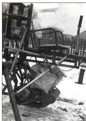
The powerplant – two IZ-P-3 single-cylinder engines mated together.
