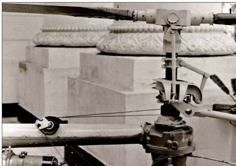
Main rotor pylon of the KhAI-27 Kharkovyanin helicopter. (Photo from the archive of Mr K. S. Gorbenko)
