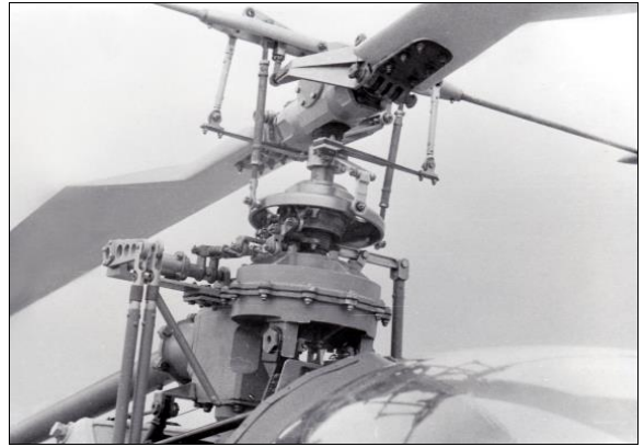
Gearbox, rotor pylon, rotor head and control system of the Va-1 helicopter.
