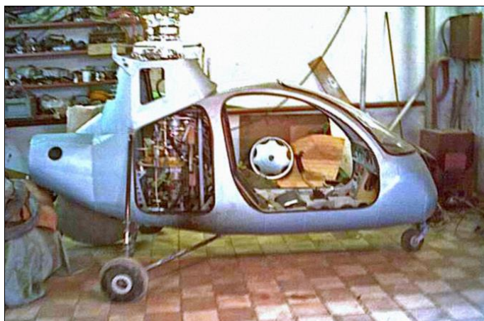
The cabin, landing gear and the powerplant of the helicopter. (Photo from the AEA Internet page)
