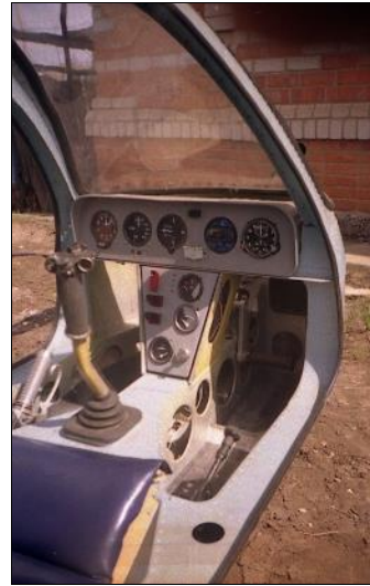
The cyclic stick and instrument panel of the helicopter. (Photo from the AEA Internet page)
