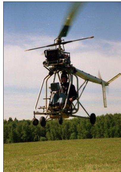
The powerplant and main rotor pylon with gearbox.
